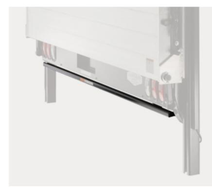
High-cycle railgates come standard with safety trip bar, auto open and close, and recessed lights. Taperintegrated cart stops are optional on extruded-aluminum platform models.
